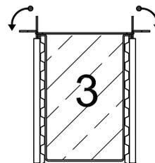
Assemble formwork units with lab joints and fix it with formbraces.
